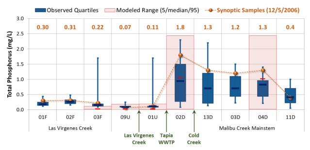
Figure 26: Modeled versus observed dry-weather Total Phosphorus at selected RSW MC Stations.
