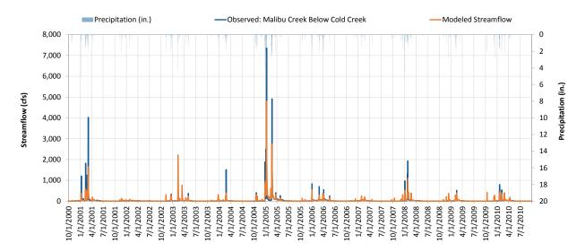
Figure 6A-5. Daily modeled versus observed streamflow at Malibu Creek below Cold Creek (F130).
