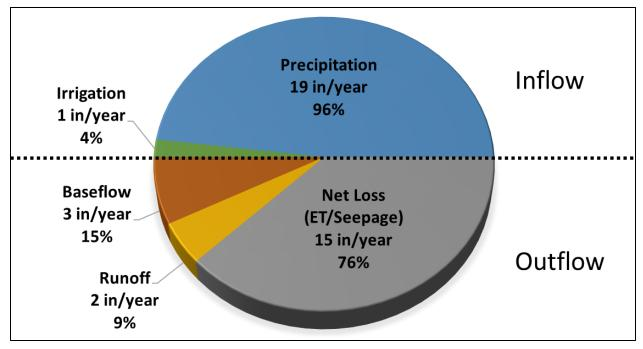
Figure 6A-3. Calibrated water balance for the Malibu Creek Watershed
