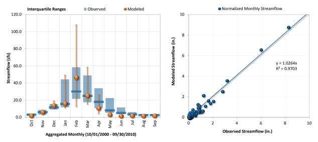
Figure 6A-8. Seasonal interquartile modeled versus observed streamflow at Malibu Creek below Cold Creek (F130).
