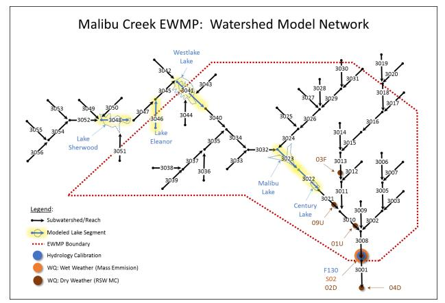
Figure 6A-1. Reach network schematic for Malibu Creek Schematic.
