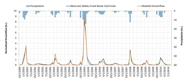
Figure 6A-6. Monthly modeled versus observed streamflow at Malibu Creek below Cold Creek (F130).
